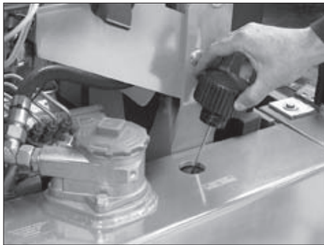
Fig. 59 Reducing residual pressure
