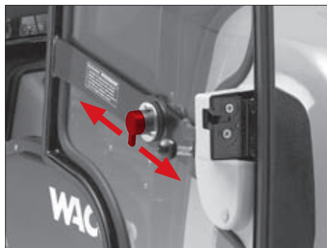
Fig. 19 Releasing locked cab doors
