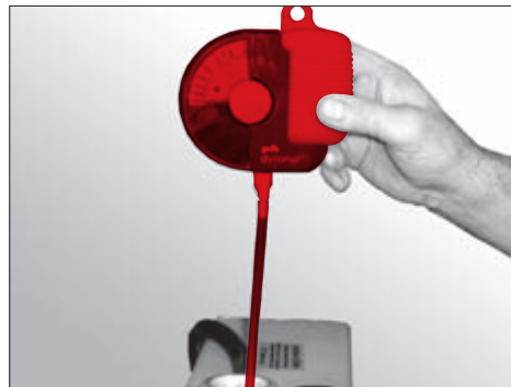
Fig. 80 Checking the anti- freeze mix
