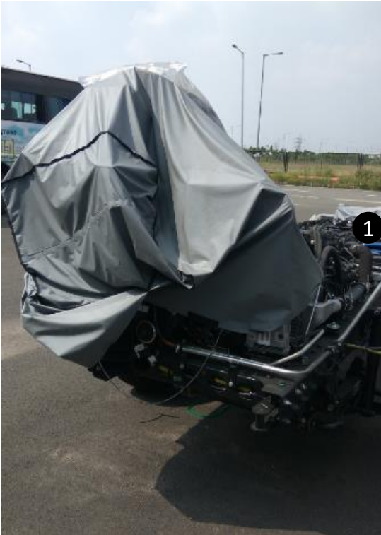
Plastic protective cover for Instrument panel and Electrical & electronic components
