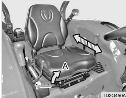
(1) Seat Adjustment Lever (A) Pull
