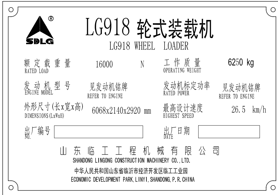
Figure 2-4 Nameplate of LG918 wheel loader mounted with long lift arms
