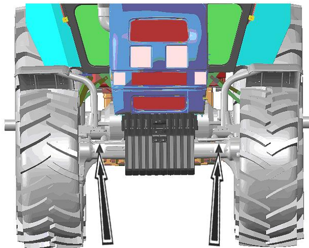
Figure 5.6.3 – Scheme of leveling jacks installation for lifting of the front elements of the tractor
