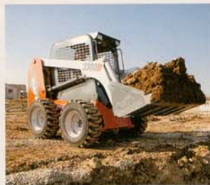
The in-line loader linkage provides excellent bucket visibility.
