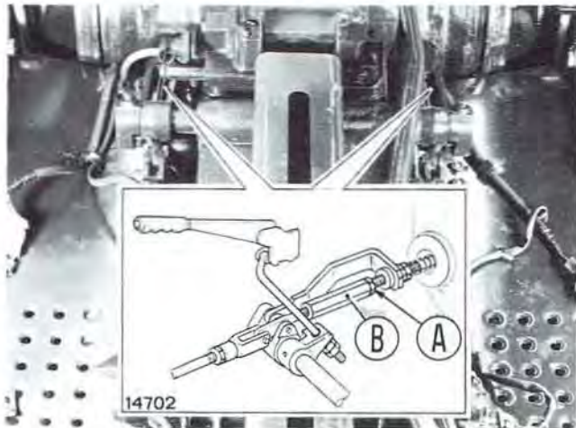
Service brake pedal travel adjustment.
