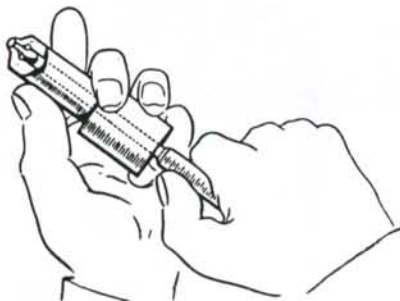
Fig. 121—Remove any carbon from dome (tip) cavity with dome cavity cleaner as shown.
