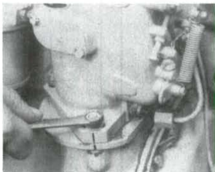
Fig. 109—View showing timing mark alignment on fuel injection pump for 1190 and 1194 models.
