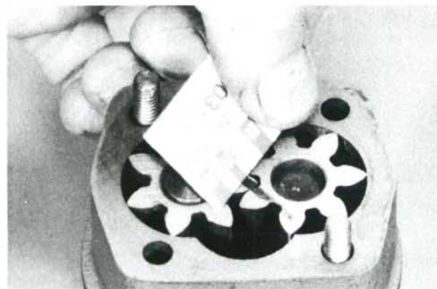
Fig. 98—View showing proper positioning of "Plastigage" when checking end clearance of oil pump rotors. Clearance must be within range of 0.025-0.089 mm (0.001-0.0035 inch).
