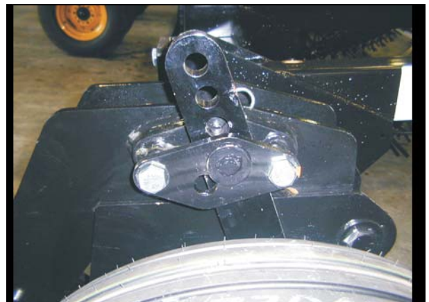
Figure 3-21 Gauge Wheel Adjustment
