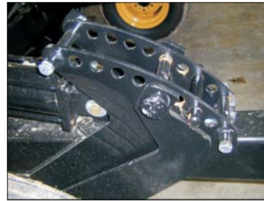
Figure 3-17 Main Frame Wheel Adjustment
