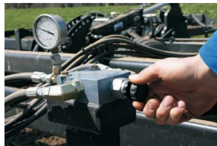
Figure 3-14 Setting Hydraulic Pressure
