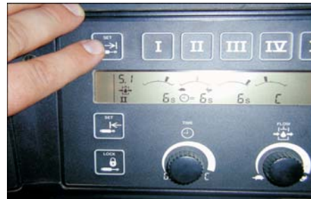
Figure 3-11 Set Valve to Slowest Position
