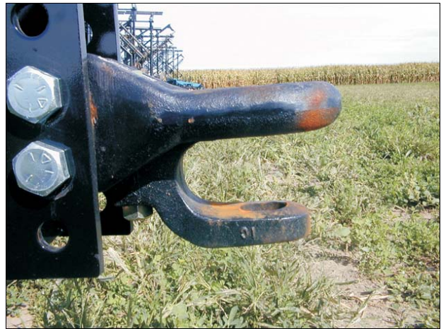
Figure 3-7 Correct Use of Double Clevis
