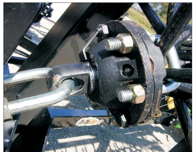
Figure 3-32 Tool Bearing Housings (12) (1 Pump of Grease Only)
