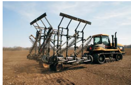
Figure 3-12 Cover Boards in Raised Position
