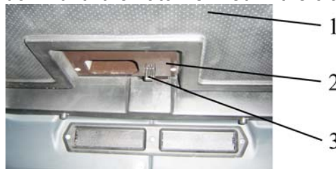
1 – hatch; 2 – board; 3 – detent.
